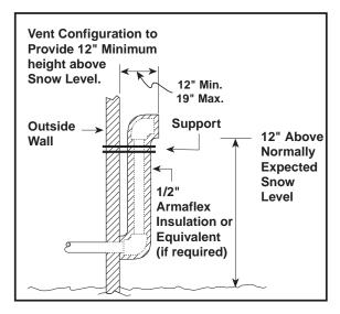
Figure 18. Alternate Horizontal Vent Installation
